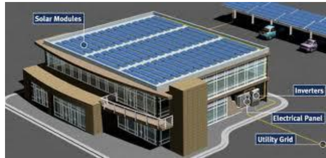
Fig. 5 Commercial Micro grid on-site
