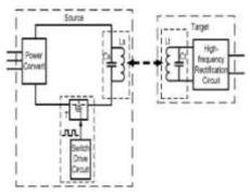
Figure 2. Block diagram of RIC
