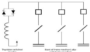
Fig 5. Schematic diagram of a SVC [3].
