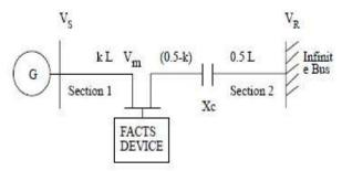
Fig 4. Series compensated transmission line with a shunt FACT device [3].
