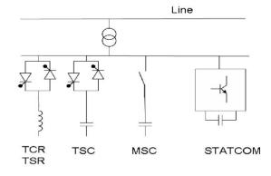
Fig 6. Examples of FACTS for shunt compensation.
