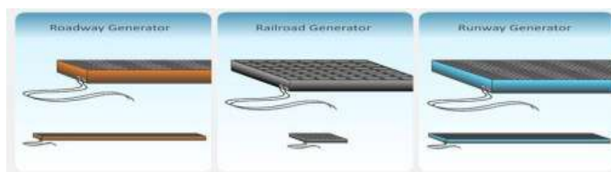
Figure 4 shows piezoelectric generator designed specifically for use in roads, places of railways, runways
