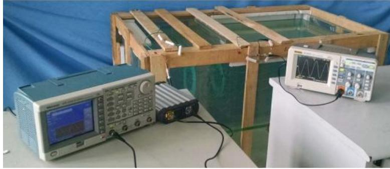
Fig. 4 Underwater WPT system experimental platform.
