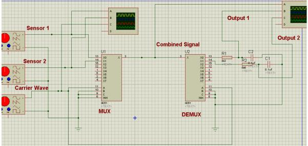
Figure 2: A simple Time Division Multiplexing (TDM) circuit designed in Proteus software
