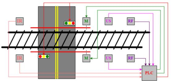
Figure 4: Schematic demonstration of the automatic operation of the system
