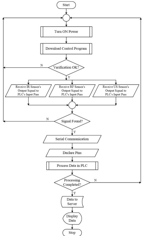
Figure 3: Flow chart of the PLC and IoT-based railway level crossing gate and track monitoring and control system
