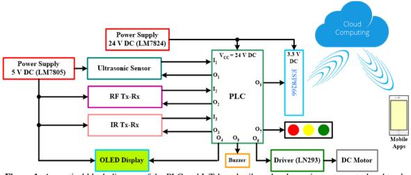
Figure 1: A practical block diagram of the PLC and IoT-based railway level crossing gate control and track monitoring system
