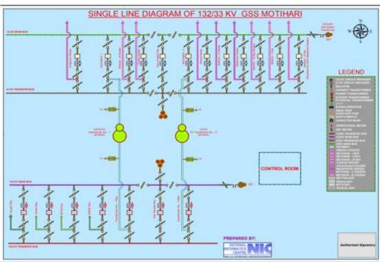
Figure 5: Single Line Diagram of the 132/33KV Grid Substation Motihari<sup>[9]</sup>
