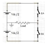
Fig. 5(a): A common half-bridge inverter
