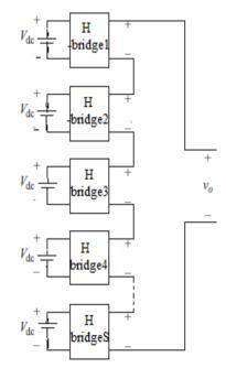
Fig.1: Multilevel Inverter with S no H-bridges.
