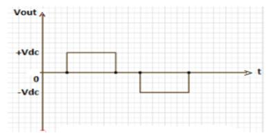
Fig.2(b). Voltage waveform of three-level inverter or a single H-bridge
