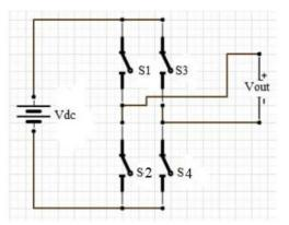
Switch ConditionOutputS1 and S4 closed+VdcS3 and S2 closed-VdcEither S1 and S3 or S2 and S4<br/>are closedOV
