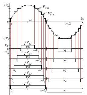
Fig. 3: Output voltage waveform of 11-level CHMLI
