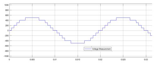
Fig. 4:Output voltage waveform of Two-level SHE-PWM inverter (without filter)
