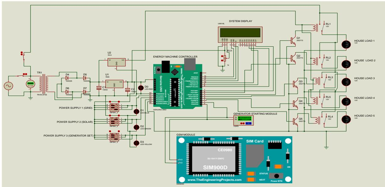
**Figure 2:** Proposed Mini-estate Intelligent Energy Machine Controller with Other Collaborative Supply Model
