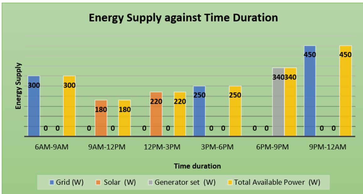
**Figure 3:** The Result of the Mini-estate Power Supply Within 24 Hours' Demonstration Period
