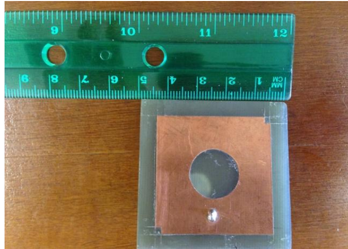
Fig. 2: Fabricated prototype of the proposed antenna
