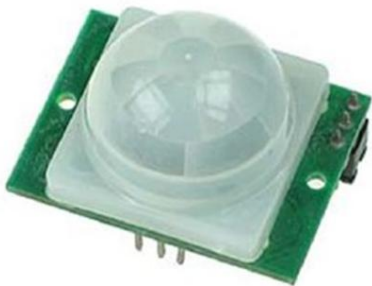
Figure 2.7 Module of PIR sensor
