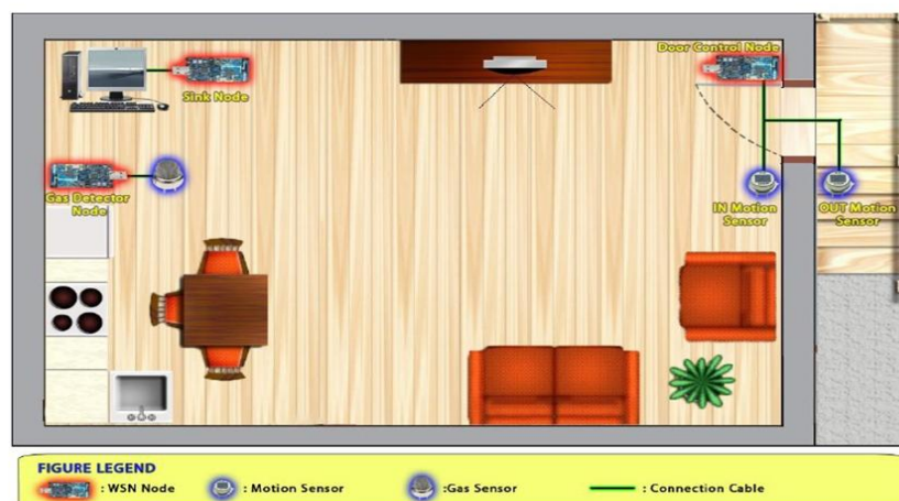
Figure 2.1 Example of layout plan for home and locations of WSN Nodes
