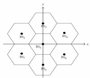
Fig. 2. Seven-cell system layout.
