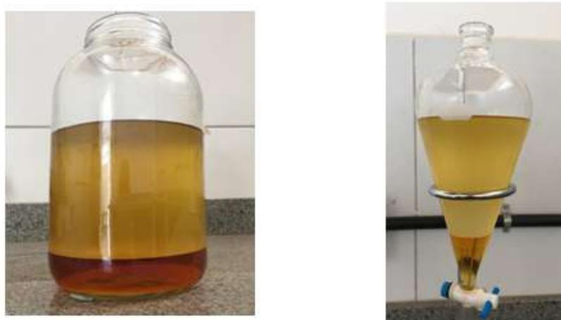
**Figure 6** – Separation between produced biodiesel and glycerin.
