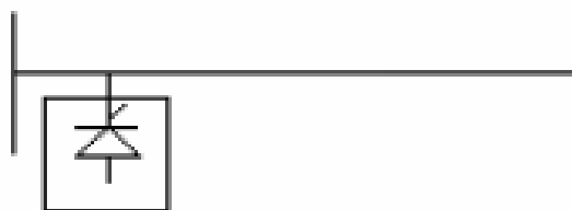
Figure: 2.2. Shunt controller
