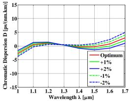
Fig.5: Chromatic dispersion curve of the PCF as a function of wavelength for first ring variation.
