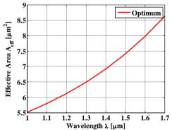
Fig.7: Effective area curve as a function of wavelength for optimum condition  $\Lambda$ =1.63 $\mu$ m, d<sub>1</sub>/ $\Lambda$ =0.332, d<sub>2</sub>/ $\Lambda$ =0.386, d<sub>3</sub>/ $\Lambda$ =0.90.
