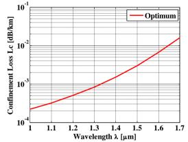
Fig.9: Confinement loss curve as a function of wavelength for optimum condition  $\Lambda$ =1.63 µm, d<sub>1</sub>/ $\Lambda$ =0.332, d<sub>2</sub>/ $\Lambda$ =0.386, d<sub>3</sub>/ $\Lambda$ =0.90.
