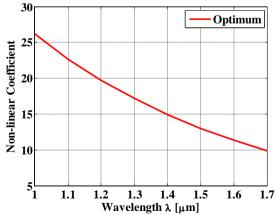
Fig.8: Nonlinear coefficient curve as a function of wavelength for optimum condition  $\Lambda$ =1.63µm, d<sub>1</sub>/ $\Lambda$ =0.332, d<sub>2</sub>/ $\Lambda$ =0.386, d<sub>3</sub>/ $\Lambda$ =0.90.
