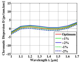
Fig.6: Chromatic dispersion curve of the PCF as a function of wavelength for second ring variation.
