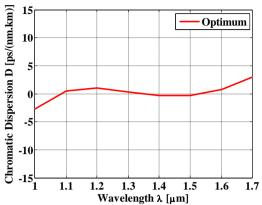
Fig.3: Chromatic dispersion curve of the PCF as a function of wavelength for optimum condition  $\Lambda$ =1.63 $\mu$ m,  $d_1/\Lambda$ =0.332,  $d_2/\Lambda$ =0.386,  $d_3/\Lambda$ =0.90.
