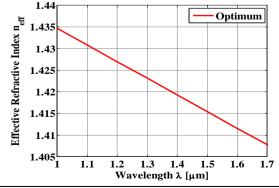
**Fig.2:** Effective refractive index curve of the PCF as a function of wavelength for  $\Lambda$ =1.63 µm, d<sub>1</sub>/ $\Lambda$ =0.332, d<sub>2</sub>/ $\Lambda$ =0.386, d<sub>3</sub>/ $\Lambda$ =0.90.
