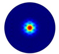
Fig.1(b): Transversal field intensity distribution at a wavelength of  $\lambda = 1550$ nm for the fundamental guiding mode of the proposed H-PCF.
