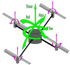
Figure. 1.1 Aerodynamic of Quadrotor
