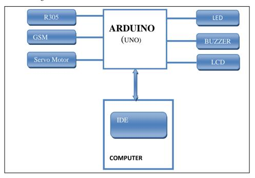
Fig 1.1A block diagram representing the circuit developed
