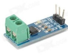
Fig. 2. ACS712 current sensor module [1]
