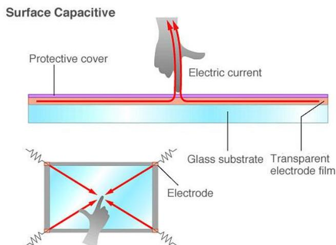
Fig.14. Layered structure of touch screen
