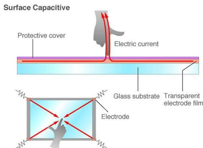
Fig.14. Layered structure of touch screen
