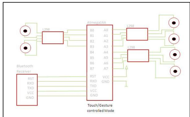
Fig.3.Simplified Schematic of touch/gesture mode
