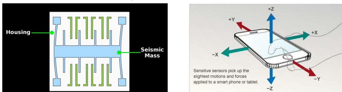
1. From the figure 15, right in the middle, there is an electrode (blue) that has enough mass to move up and down very slightly when movement or tilt is produced.
