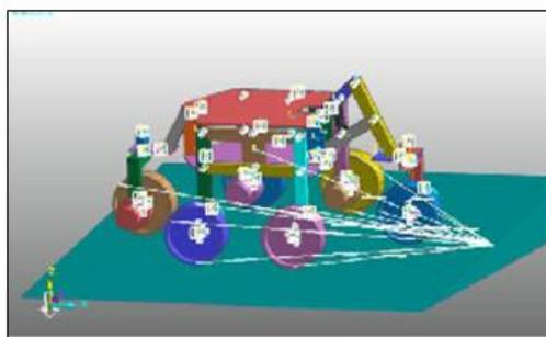
Fig.7. Shrimp rover model in RecurDyn
