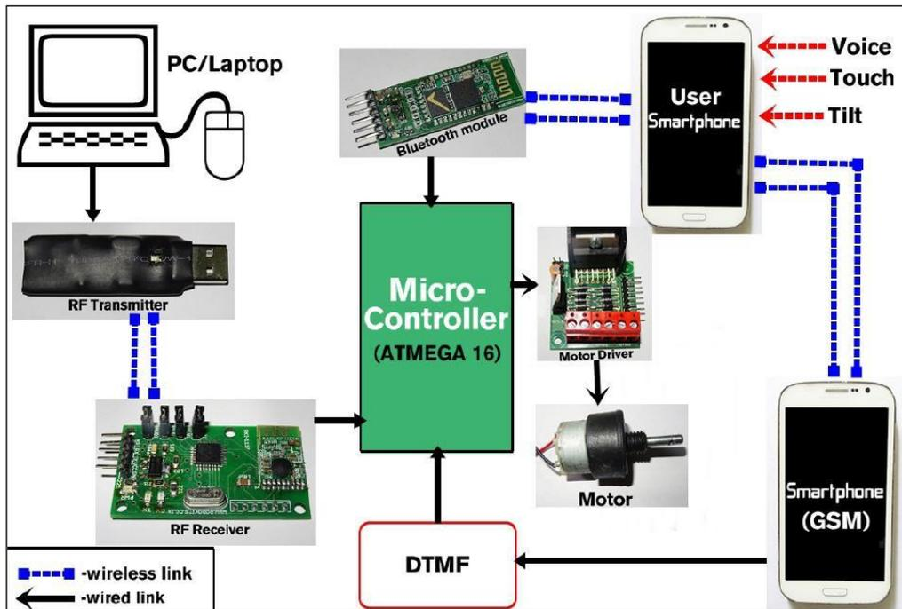
Fig.1. Main Block Diagram
