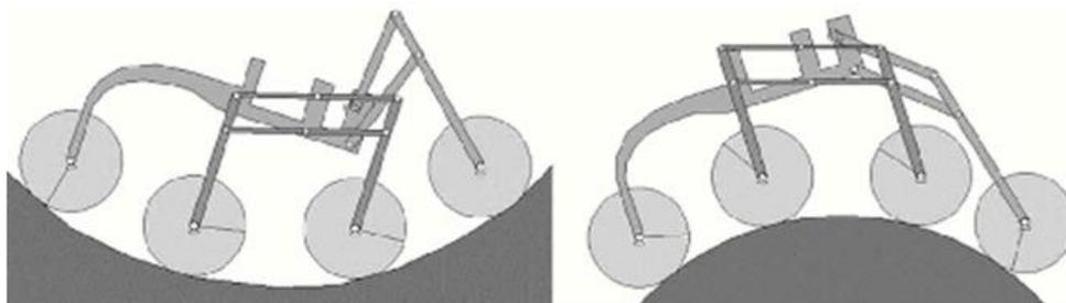
Fig.6. Structure on concave and convex ground
