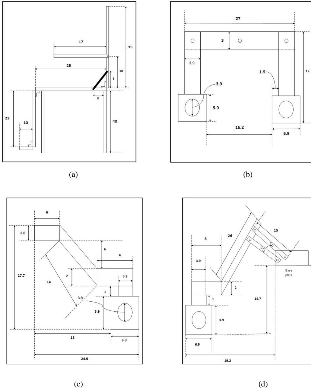
Fig.5. Mechanical Design (a) Chair dimension (b) Centre bogie (c) Rear fork (d) Front fork
