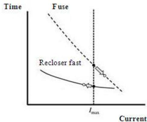
b) The impact of DG on coordination between the fuse and the recloser (fast-mode)
