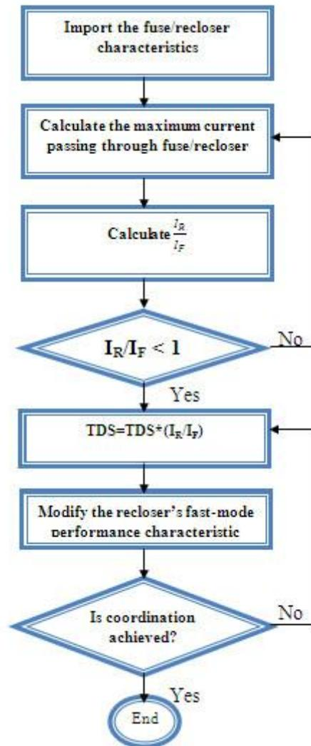
Fig. 5 Flowchart of adaptive relay for recloser-fuse coordination protection scheme
