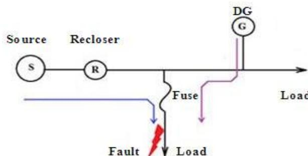
a) A feeder with one recloser, one fuse, and one DG source
