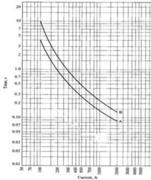
Fig. 1 MMT characteristic (A) and MCT characteristic (B) of a given fuse
