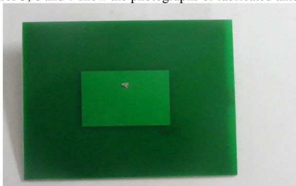
Figure 5 Photograph of Fabricated Microstrip antenna
