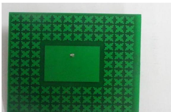
Figure 6 Photograph of Fabricated Microstrip antenna with EBG structure without vias
