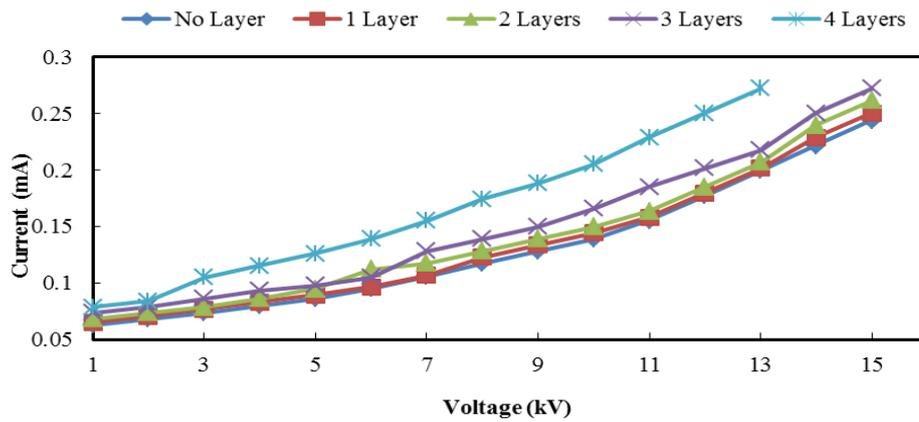
Fig. 6: Leakage current as a function of applied voltages when different layers of insulation papers are held between the electrodes in oil with 25 ppm DBDS concentration.
