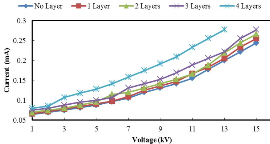
**Fig. 9: Leakage current as a function of applied voltages when different layers of insulation paper are held between the electrodes in oil with 25 ppm DBPC concentration.**
