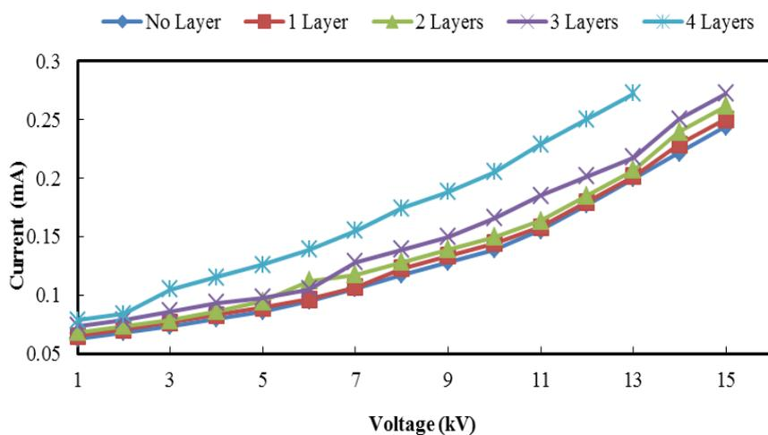
Fig. 7: Leakage current as a function of applied voltages when different layers of insulation paper are held between the electrodes in oil with 50ppm DBDS concentration.
