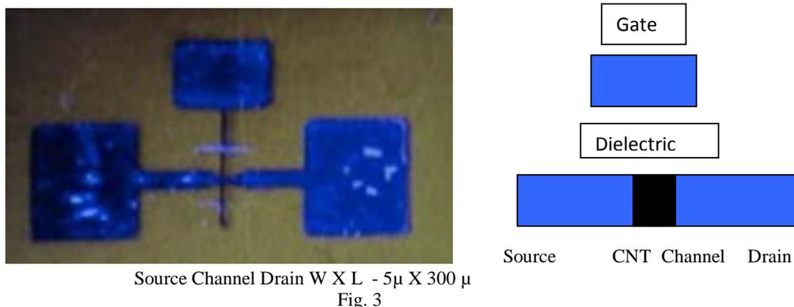
Source Channel Drain W X L -  $5\mu \times 300\mu$
