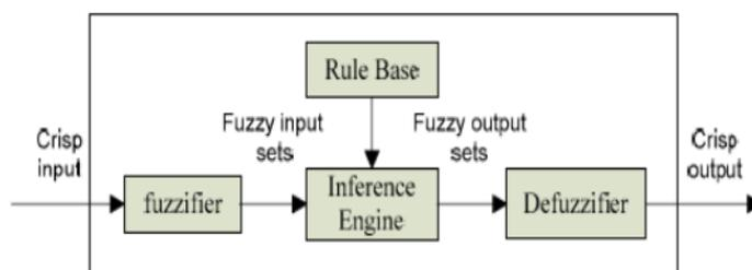
Fig.3.General architecture of fuzzy logic system (FLS)
