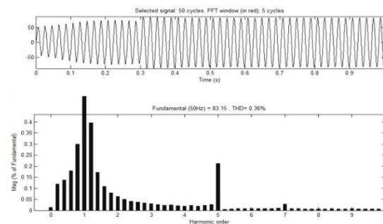
Fig.7.FFT of source current with STATCOM
