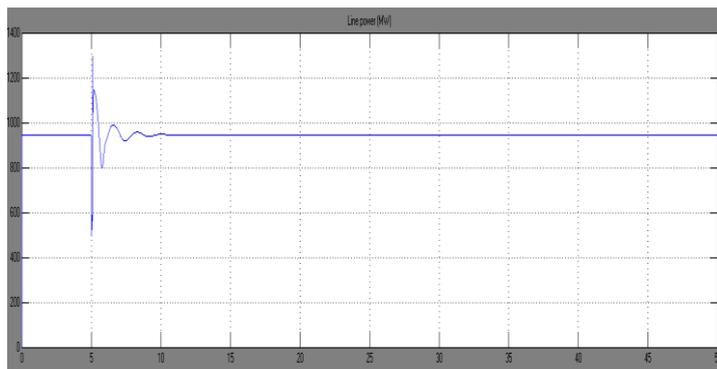
Fig.13 (b) transmission line active power of the system when Fuzzy logic control is used for SVC
