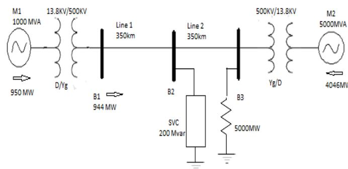
Fig.7. Single Line diagram of 2-Machine 3-Bus system
