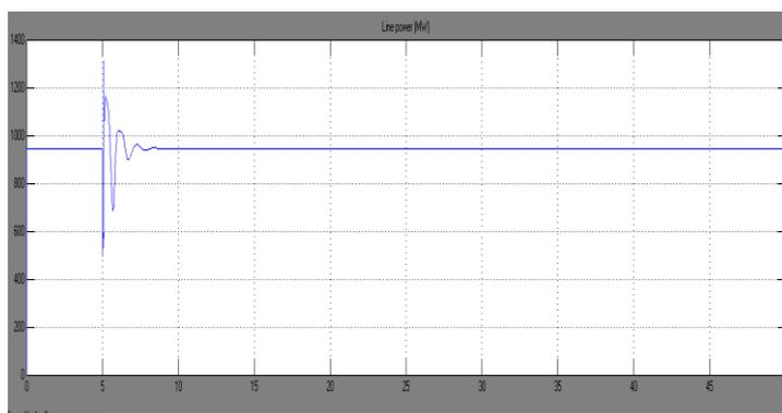
Fig.13(c) transmission line active power of the system when PI-Fuzzy logic hybrid control is used for SVC
