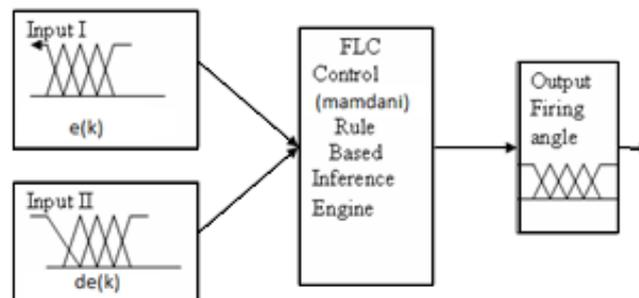
Fig.6. Structure of Fuzzy Logic Controller
