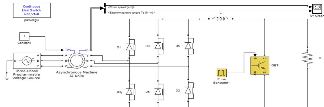
Figure 1: Wound Rotor Induction Motor employing pulse generator
