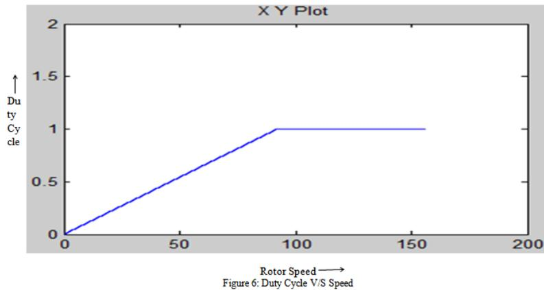
Figure 6: Duty Cycle V/S Speed
