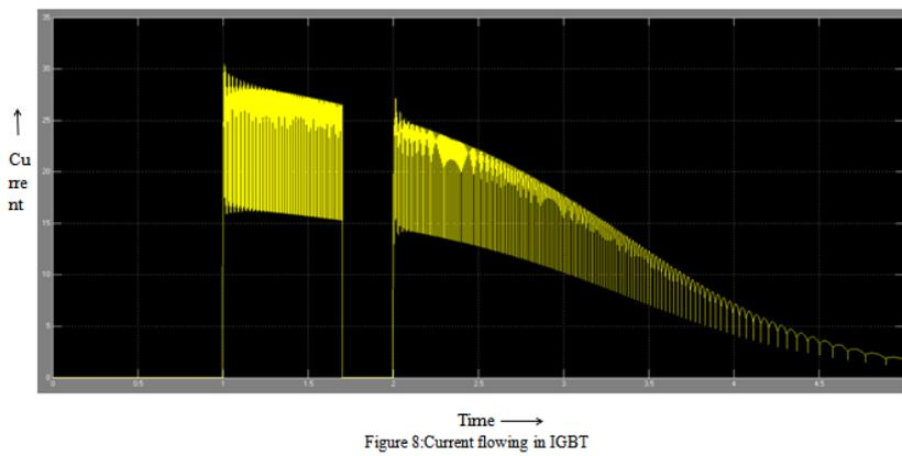
Figure 8: Current flowing in IGBT
