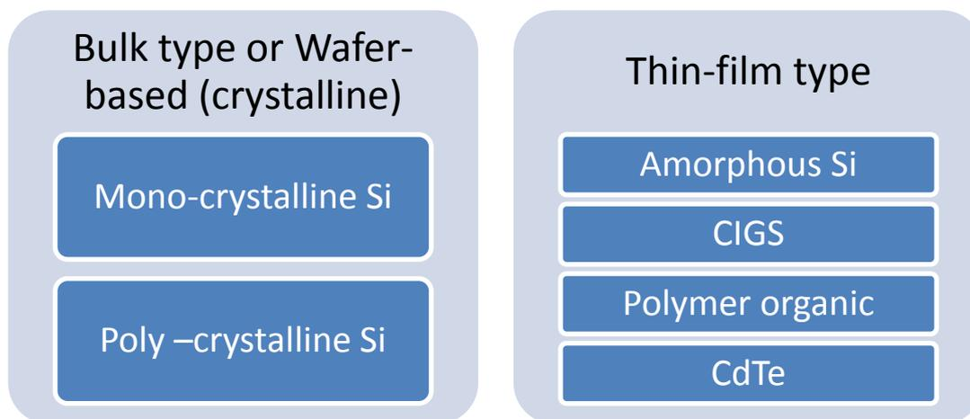
Fig. 2 classification of solar panels
