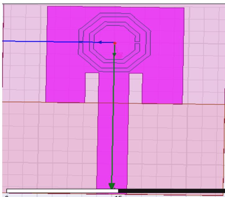
**Figure 3:** Antenna in the presence of single unit cell.
