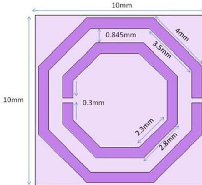
**Figure 2:** The unit cell structure and its dimensions.
