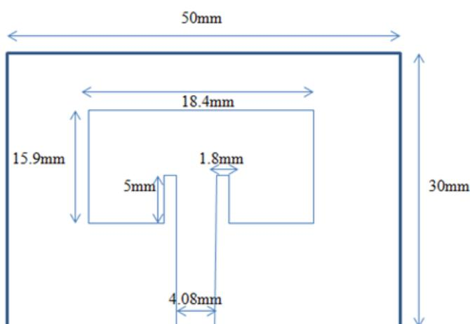
Figure1: Basic structure of conventional rectangular MPA.
