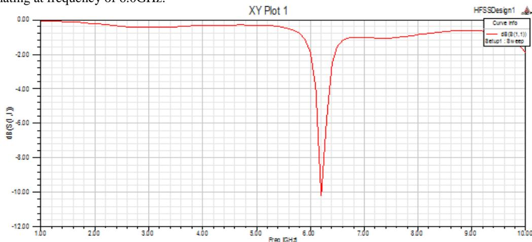
Figure 4: Return loss of conventional antenna.
