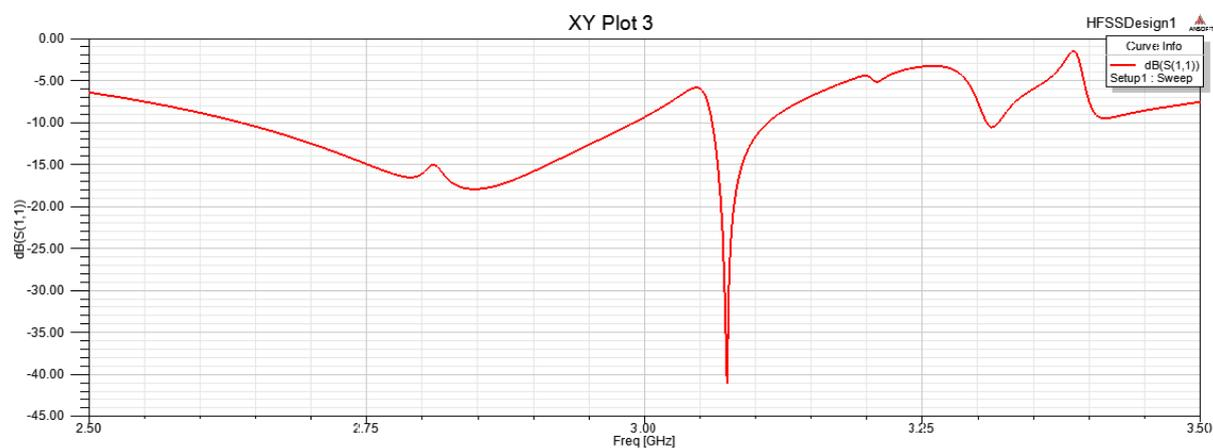
Figure 5: Return loss of proposed antenna
