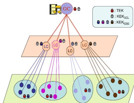
Figure (2): The group key generation and distribution in BALADE.
