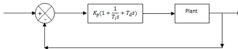
Fig.1 Design of PID control of plant
