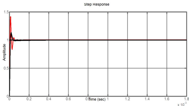
**Fig 5.** Unit step response of the monotonic compensation (dashed line) and the non-monotonic compensation (solid line).
