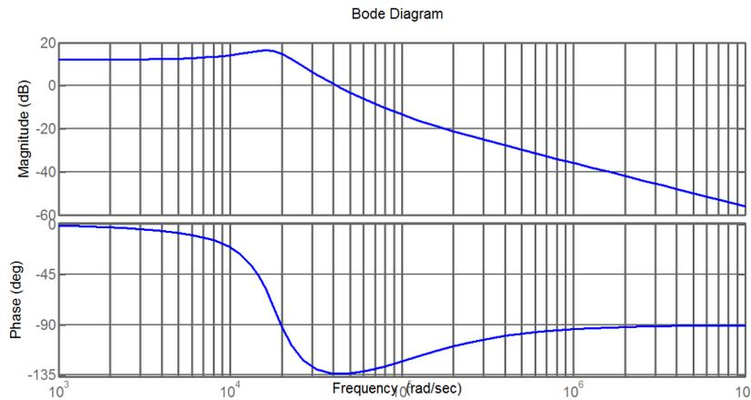
Fig.2 Bode plot for Buck regulator
