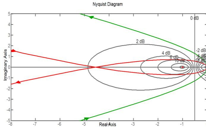
**Fig 4.** Nyquist plots for the monotonic compensation (dashed line) and the non-monotonic compensation (solid line).
