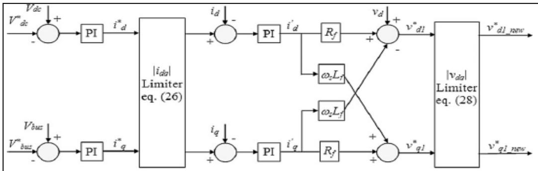
Figure 4.1 : Direct-current vector control structure of the GSC.
