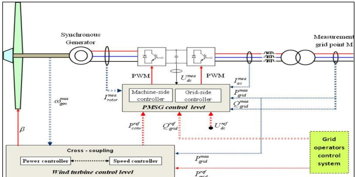
Figure 2.1: Configuration of a Permanent Magnetic Synchronous Generator wind turbine.
