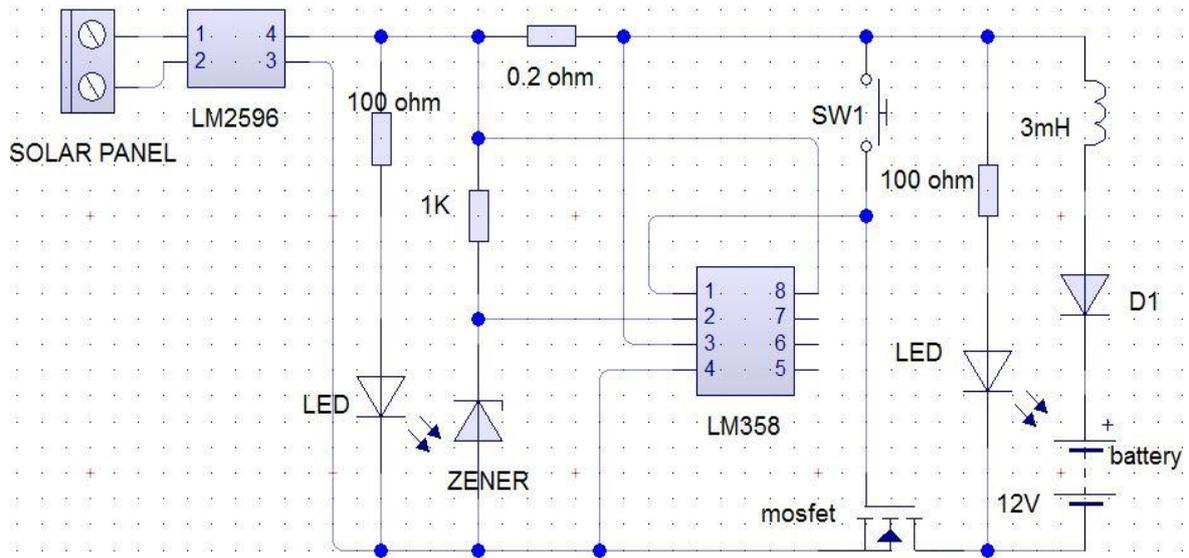
Fig.4: Complete diagram of cost efficient solar PV charge controller
