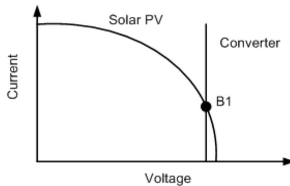
**Fig.1:** Characteristics of PV voltage controller
