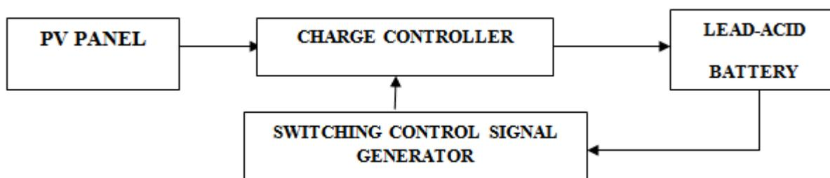
**Fig.2:** Simplified Hardware Block Diagram of a Solar Charging Station
