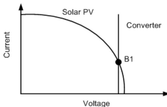
**Fig.1:** Characteristics of PV voltage controller
