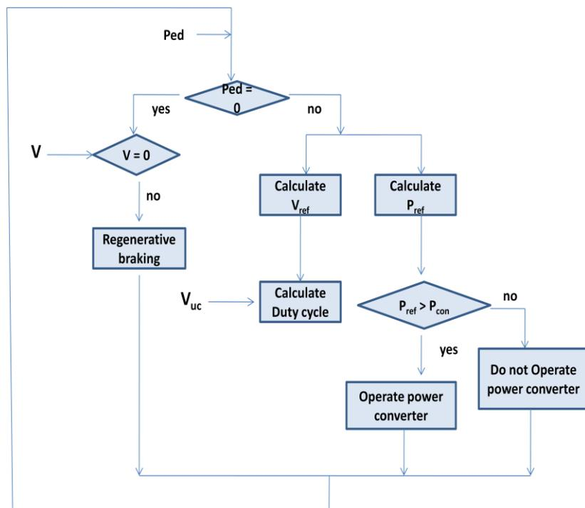
Fig.3. Flow chart of the outline of control algorithm
