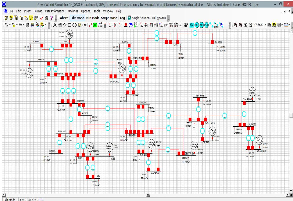
Figure 4: Existing 330KV transmission network with scheduled load in the PWS Edit mode
