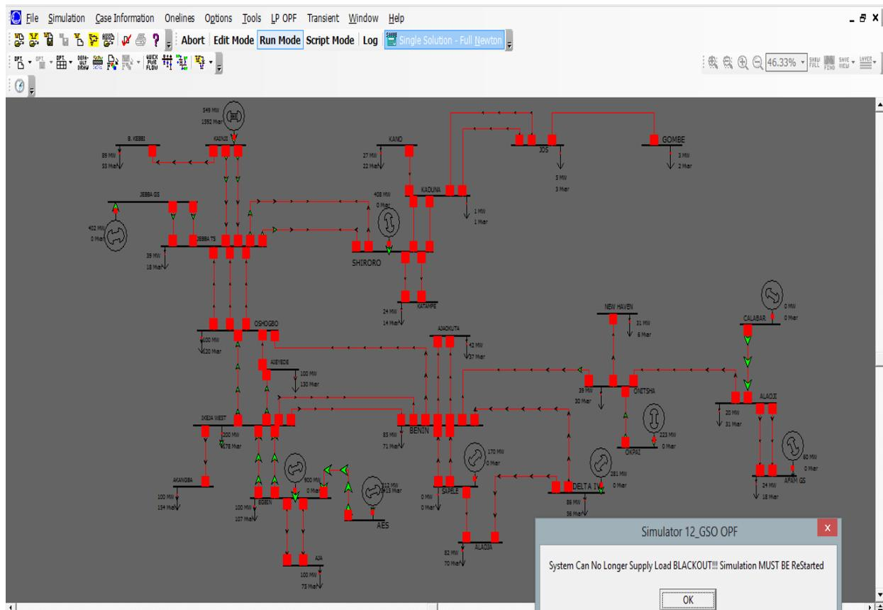
Figure 6: Blackout occurring when simulation is solved
