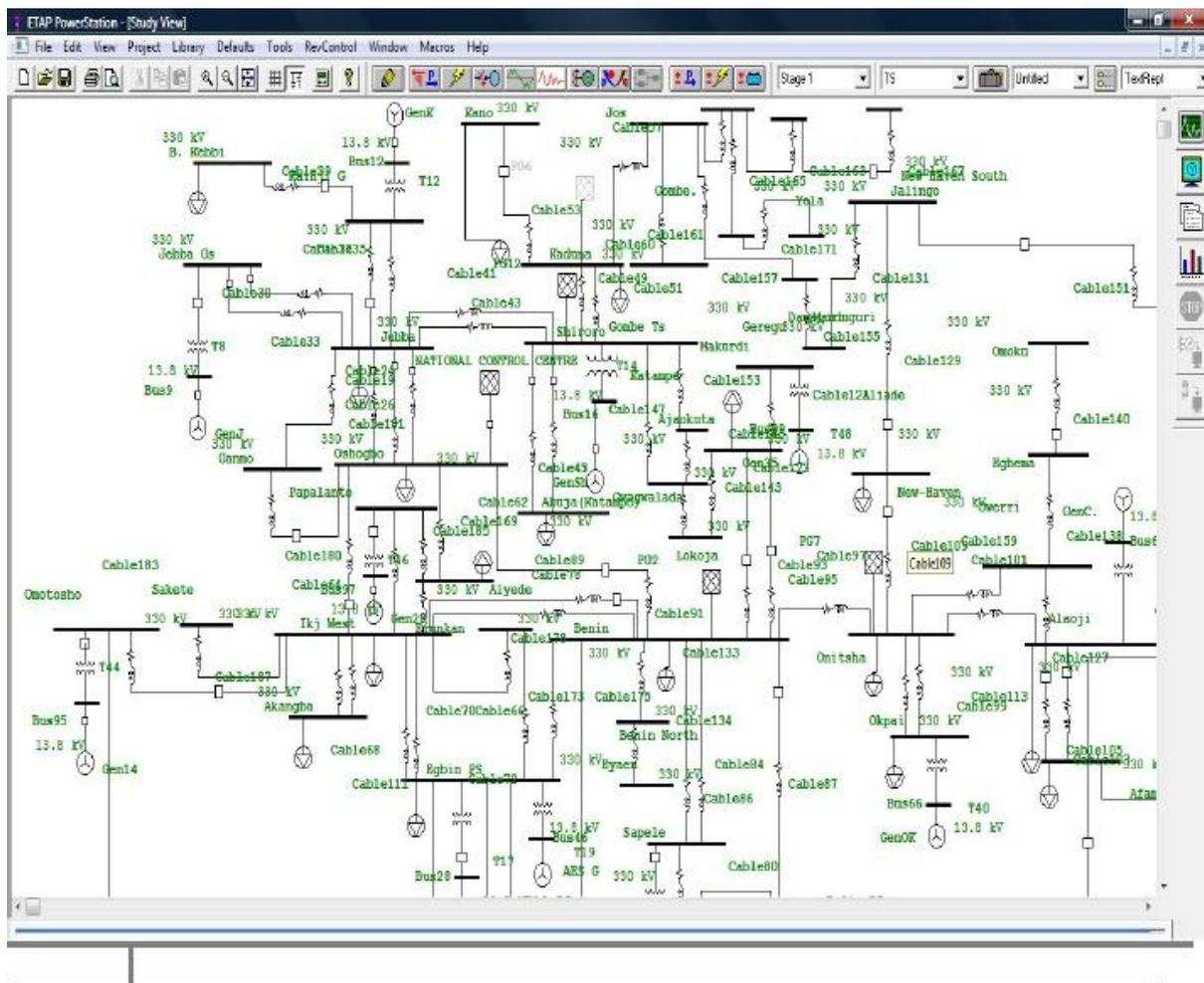
**Figure 3: Existing 330KV Nigeria Transmission Network**
