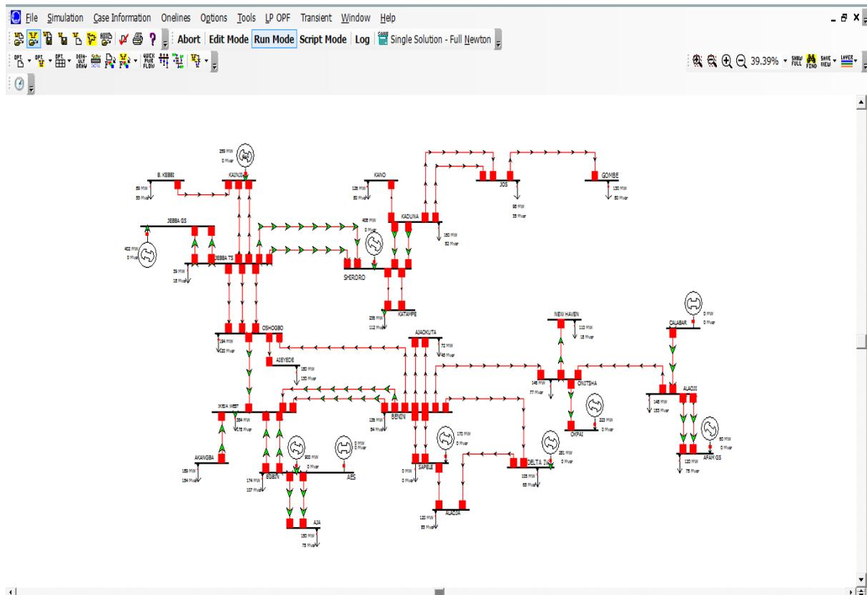
Figure 5: Existing generation with estimated actual load demand in run mode
