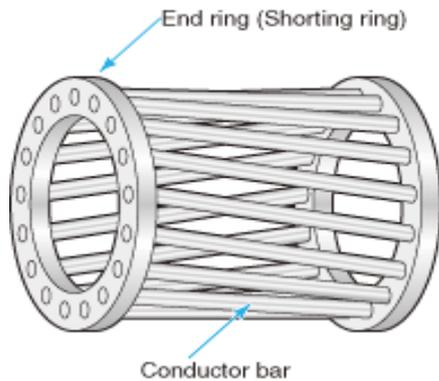
Fig2:Squirrel Cage rotor
