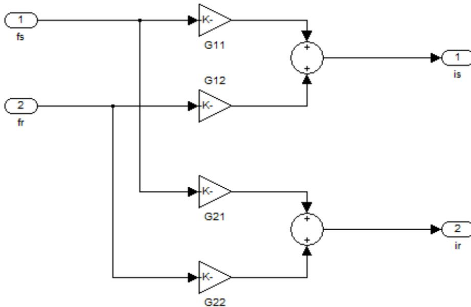
Fig16: Model for flux current relations
