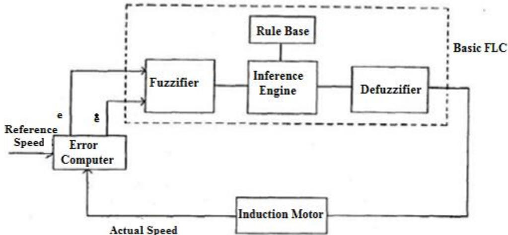
Fig 5:Block diagram of a Fuzzy Logic Controller
