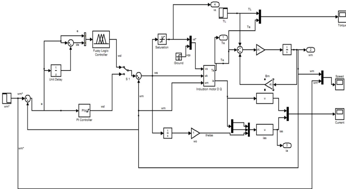
Fig18:Matlab/Simulink Model of Fuzzy Controller
