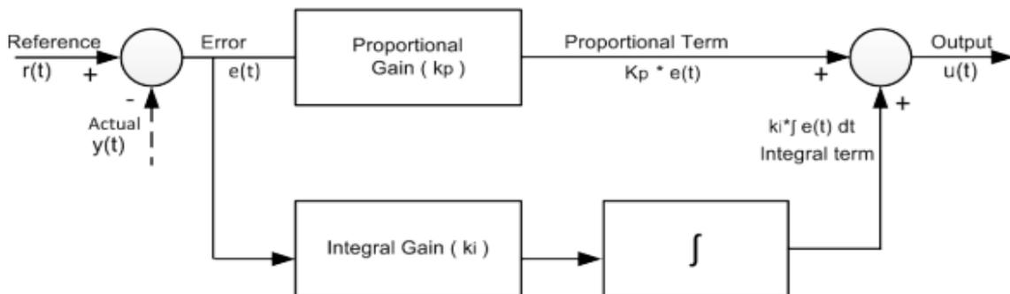
Fig 4: PI Controller block diagram.
