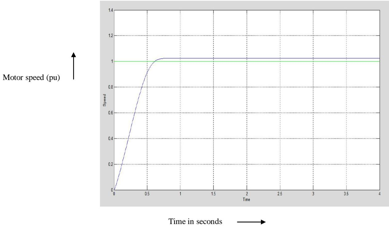
Fig 17: Speed V/S Time Response of PI controlled Induction Motor
