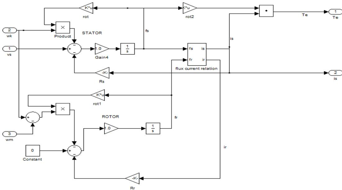
Fig15: Space vector model of Induction Motor
