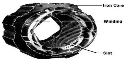
Fig1: Stator of an Induction Motor
