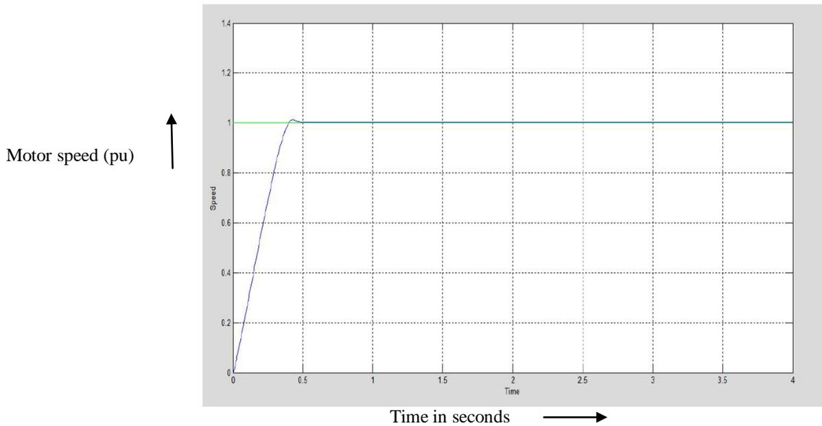
Fig 19: Speed V/S Time Response using Fuzzy logic controller
