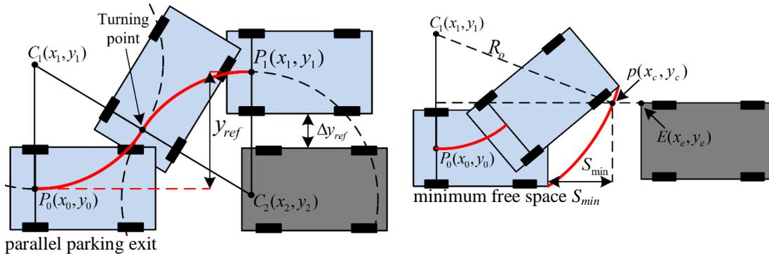
Fig. 5 parallel parking exit for one maneuver case
