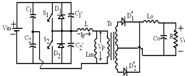
Fig.3 Half bridge LC filter circuit
