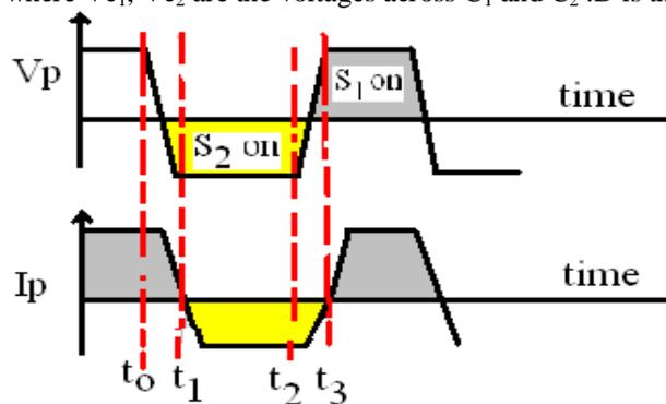
Fig.4 Half bridge APWM waveforms
