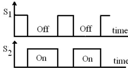
Fig.2 Gate pulse for APWM control
