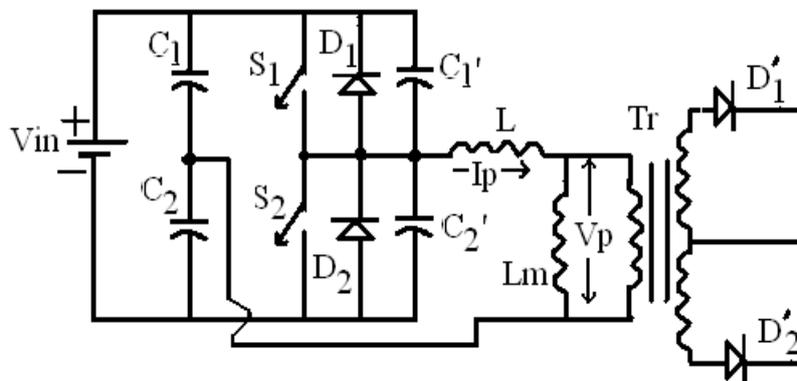
Fig.1 Half bridge ZVS-Clamped voltage configuration
