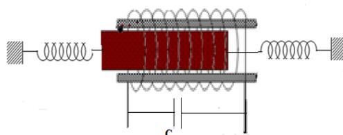
Figure 3 LOTM with return springs and the ability to stop by electrical damping
