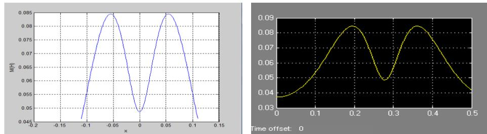
Figure (11.a, 11. b). Variation of the mutual  $M$  in function of the displacement and the time
