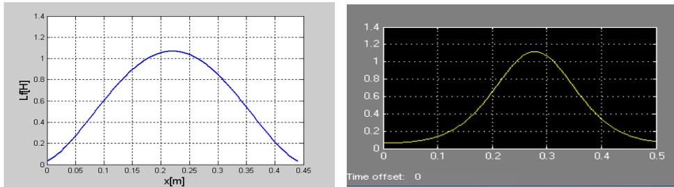
Figure (8.a, 8. b) Variation of the inductance of the nucleus  $L_f$  in function of time and displacement.
