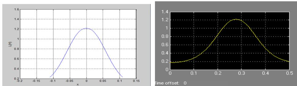
Figure (10.a, 10. b) Variation of the total inductance  $L$  in function of the displacement and the time
