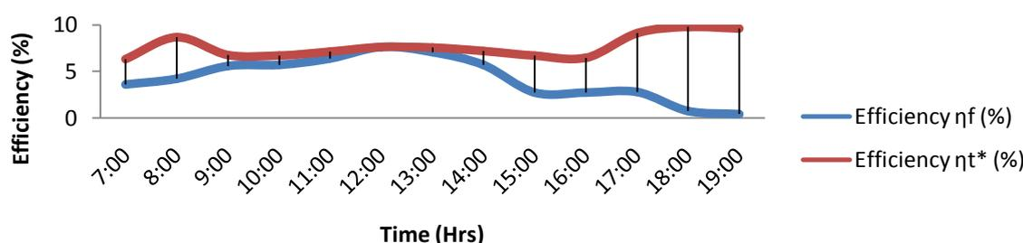
Figure 3: Efficiency comparison between fixed and tracking pane
