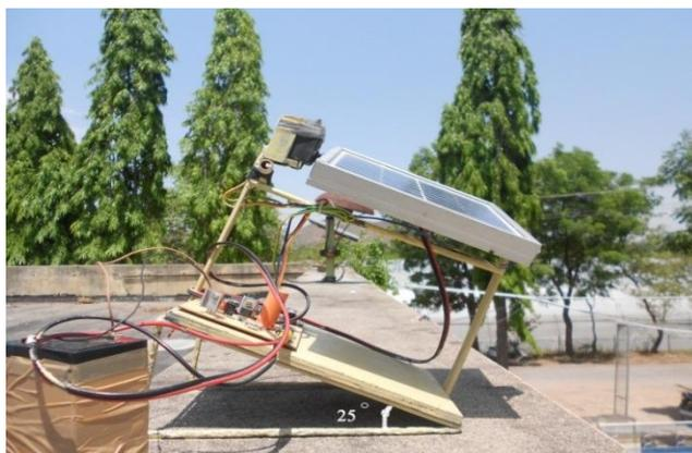
Figure 4: Developed tracking system
