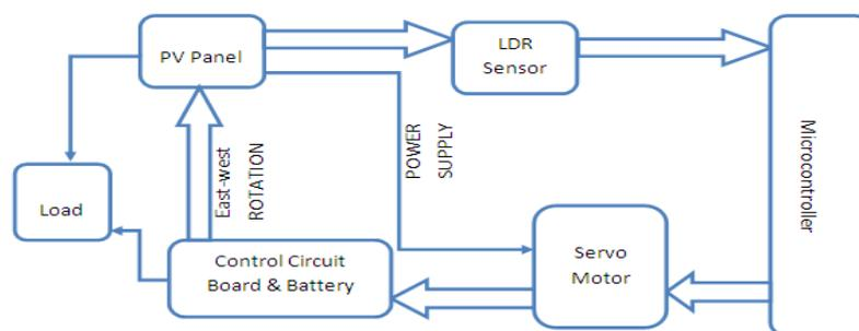
Figure 3: Block diagram for working of tracking mechanism
