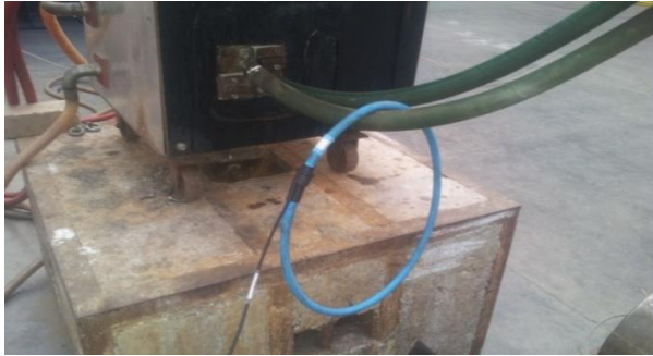
Fig.14 application of rogowski coil for induction heating
