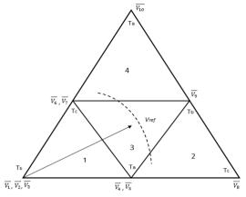
Figure.6 Voltage vector I and their times in sector I TABLE 3 TIME CALCULATION FOR REF V IN SECTOR I
