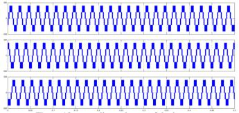
Figure.12 output line voltages of the inverter
