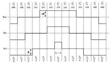
Figure.8 switching sequence of thirteen segments for  $V_{ref}$  in sector-I of region-1
