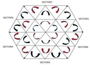
Figure7.Switching sequence for three-level SVM inverter
