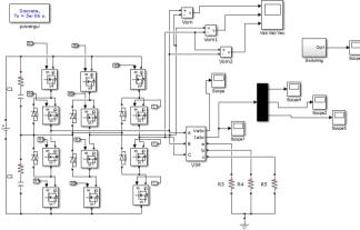
Figure 9. Three-level diode clamped Multi-level inverter
