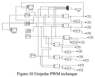
As per the principle of unipolar pwm three reference sine and two carrier waves are compared as shown in figure.2 for pwm signals. The generated signals are as shown in figure 11.
