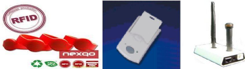
Fig.4 Wristband tag, PC-Card Reader and the Smart Field Generator [10][11][12]
