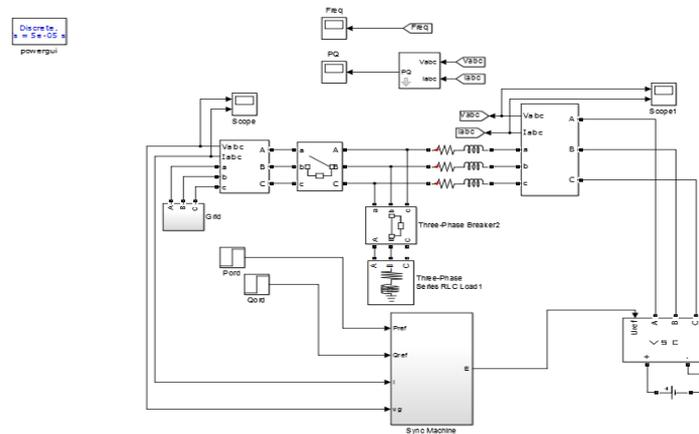
Fig :4 Simulation of synchronverter
