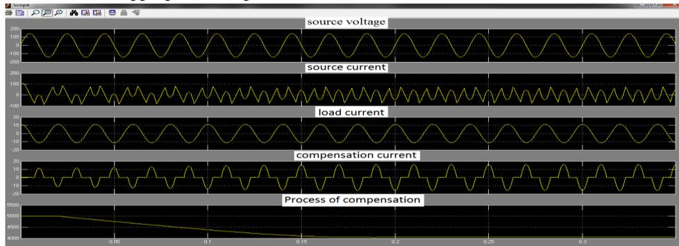
Figure.7 Source voltage, line current, load current, compensation current and process of closed loop compensation of TCR circuit.
