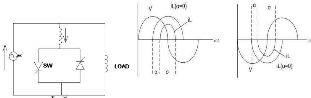
Figure 4. Basic Thyristor-controlled reactor (TCR) firing Delay Angle Control and operating waveform
