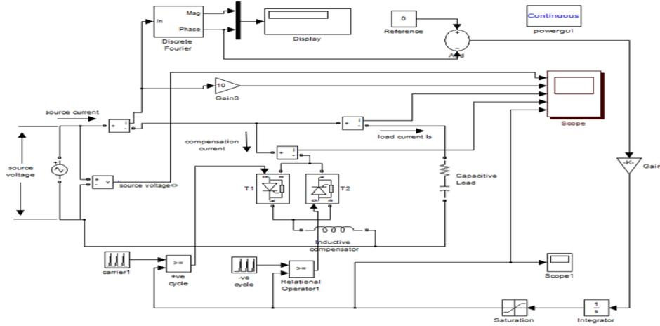
Figure.6 Circuit Configuration of TCR
