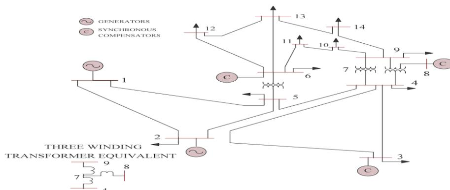
Figure-8.IEEE 14-bus benchmark test system.
