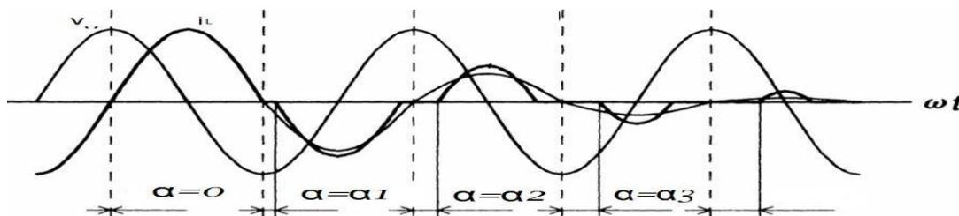
Figure 5. Operating waveform of TCR
