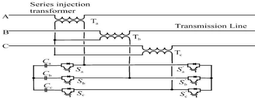
Figure no.1 Transmission line with PWM SVeC.
