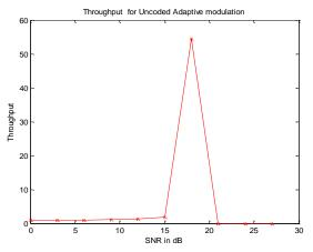
Figure 6. Throughput of Uncoded AOFDM with BPSK, QPSK, QAM
