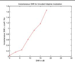
Figure 3. Instantaneous SNR of Uncoded AOFDM with BPSK,QPSK,QAM
