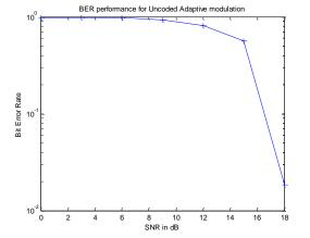
Figure 2. BER Performance of Uncoded AOFDM with BPSK,QPSK,QAM
