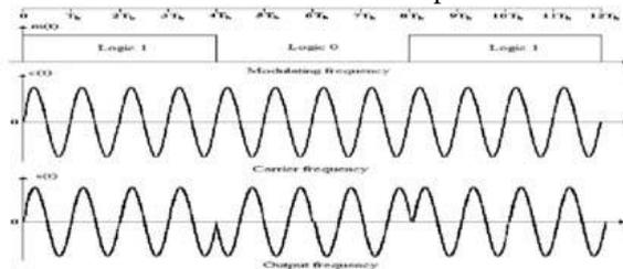
**Fig. 2: BPSK waveforms**
