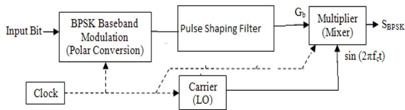
**Fig. 1: BPSK transmitter using FPGA BLOCK DIAGRAM**
