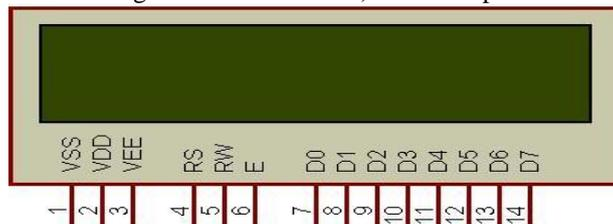
Figure 5 Character LCD type HD44780 Pin diagram
