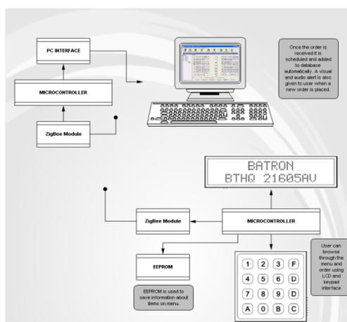
**Fig.1 Basic Block diagram of Automated Restaurant Using ZIGBEE Module**
