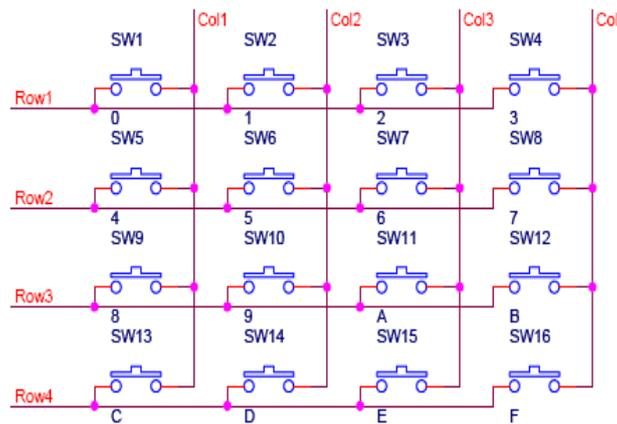
Fig.3. Keypad Using SPST.
