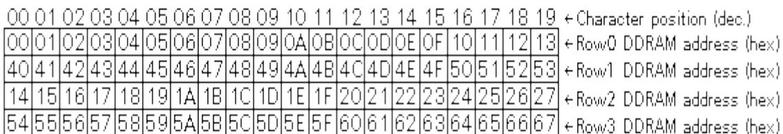
**Figure 8** DDRAM Address for 4 Line LCD
