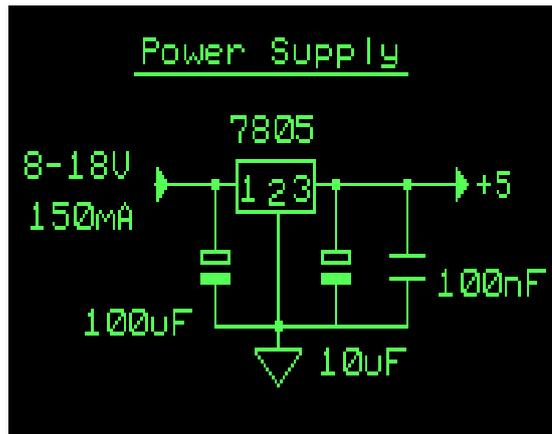
Fig 9 Circuit diagram of power supply.
