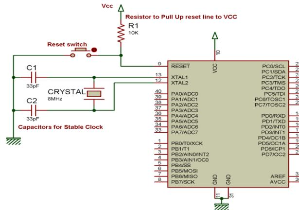
Fig 4. Circuit For AVR Microcontroller
