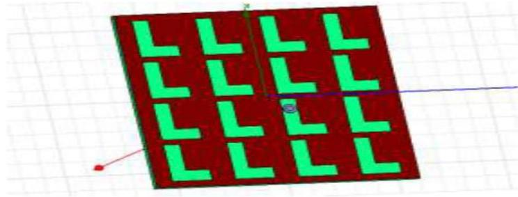
Fig.7: Circular Patch Antenna with L-shape DGS
