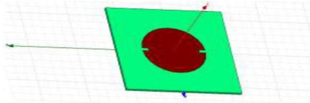
Fig.1: Circular Microstrip Antenna
