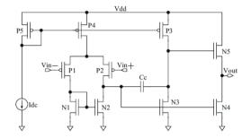
Fig.4. Three stage op amp with PMOS input transistors
