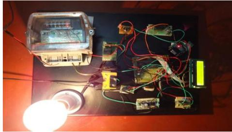
**Stage 2:** The meter detects the number of pulse consumed by the load and display on the LCD.
